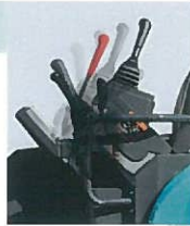
All operations are blocked when the lever is raised.
